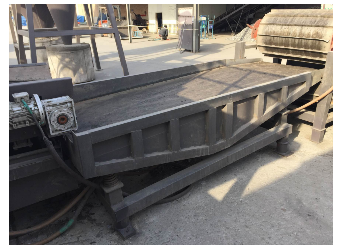
Discharging vibration equipment
